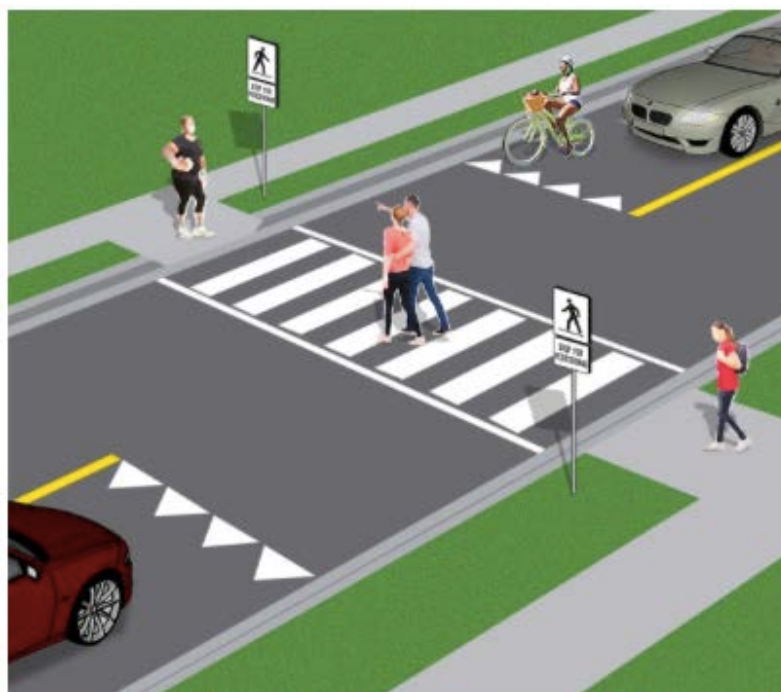
Figure 17. Example of a pedestrian crossover that could be modified for V2I use
